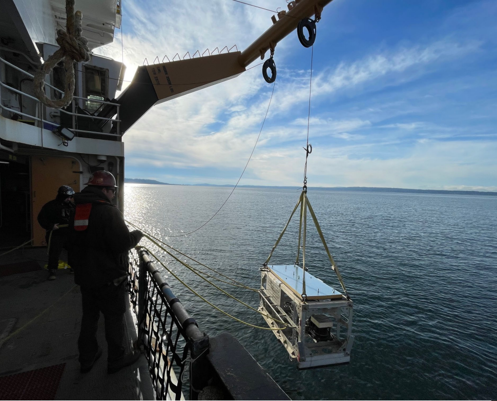
Experimental Low Frequency (ELF) transducer testing to investigate pollock size classification (Shumagins)
