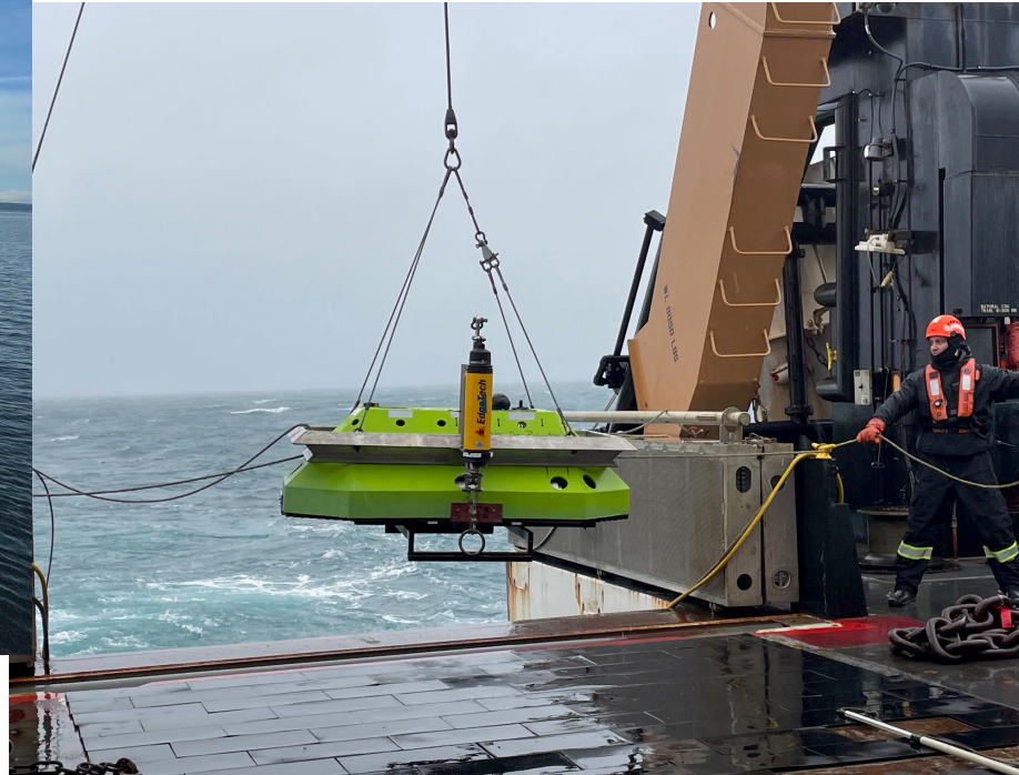
Deployed transducer/hydrophone mooring in Shelikof to investigate pollock vocalizations during spawning (Shumagins)
